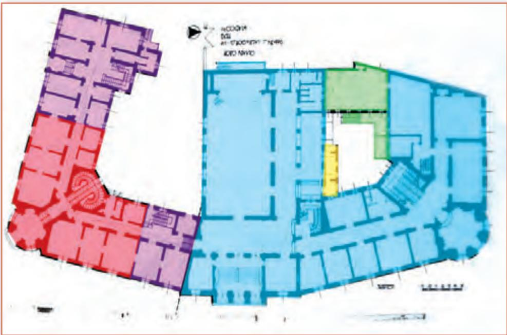
**Fig. 10.** Scheme of the stages of construction of the building: Stage I - red; stage II - violet; stage III - blue; stage IV - green; stage V - yellow
